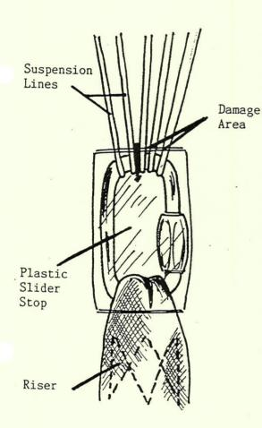
It has come to our attention that some canopies are suffering damage to suspension lines, particularly canopies with micro-line. The damage is occuring near the attachment point to the connector link or level with the slider stops.
