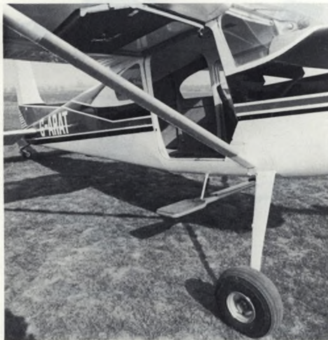
The only 'in flight' door in the country having just been fitted to John Meacock's Cessna 180 at Sibson — warm flights and fast climbs are the result. photo Nick Cullum
