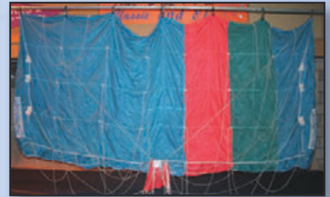
A pull-up cord left in and an incorrect bridle routing
