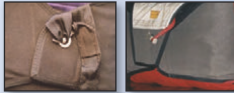
A pull-up cord left in and an incorrect bridle routing
