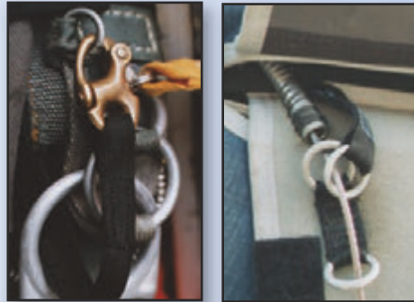
Both RSLs are routed incorrectly – would you spot it or do you just know how yours works?
