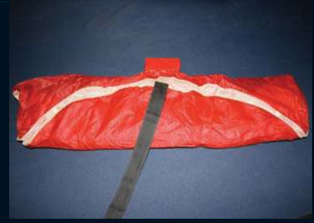
Neatly laying the excess line in the container
