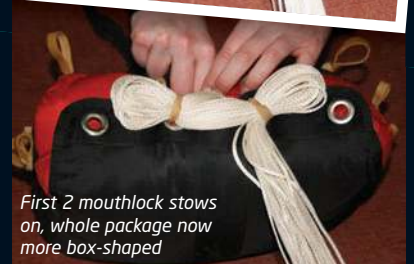
Rolling the mouthlock bungee to the grommet, using technique and bodyweight over brute strength
