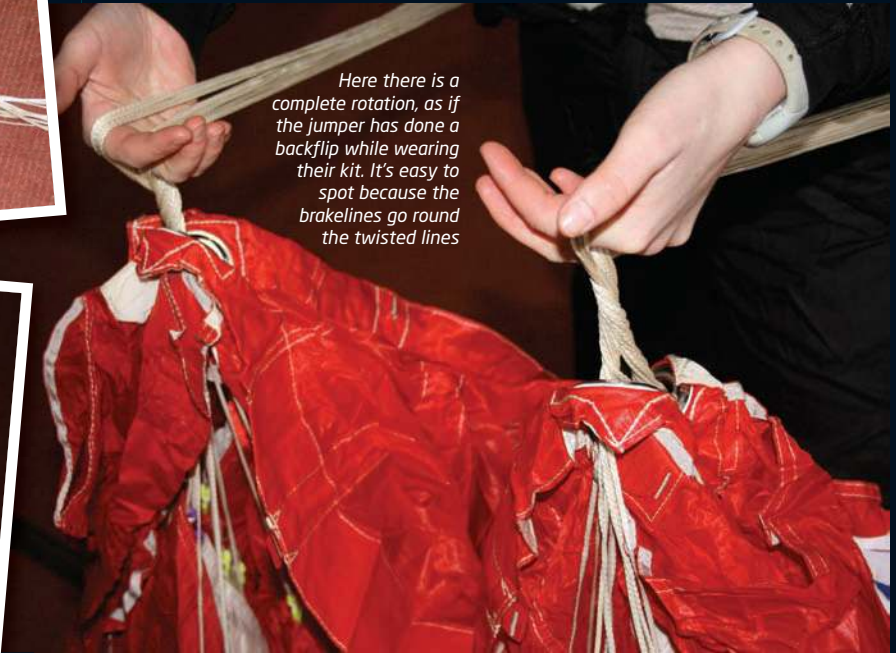
Separate the front left riser and rear left riser line groups and the left brakeline. Now walk up to the canopy, letting the lines run through your fingers
