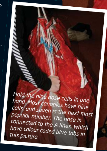
The canopy is now ready to place on the floor in a controlled manner. Notice the lines are still taut
