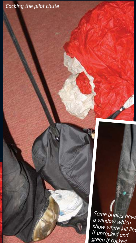
Now the pilot chute is cocked, most of the kill line has gone back inside the bridle
