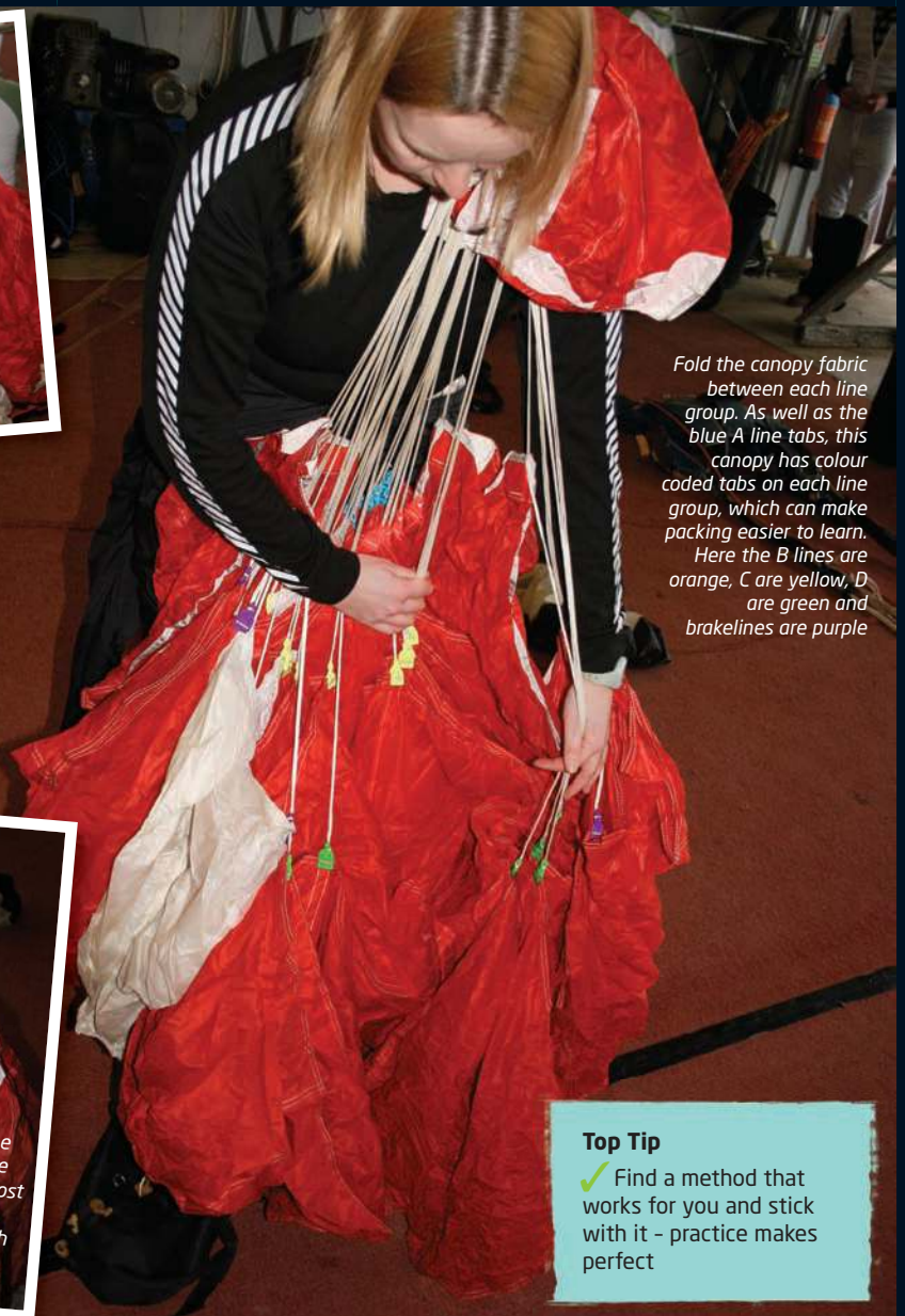
The canopy is now ready to place on the floor in a controlled manner. Notice the lines are still taut
