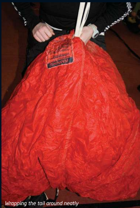
The canopy is now ready to place on the floor in a controlled manner. Notice the lines are still taut
