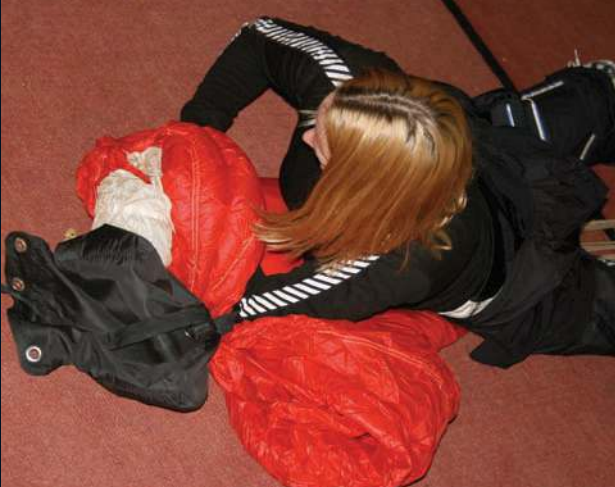
Squashing the air out and gently folding the canopy to the correct width
