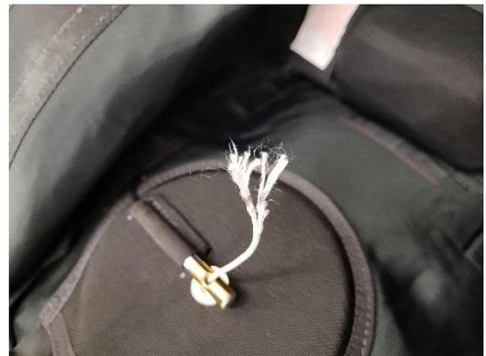
During the inspection, no sharp grommets or edges to the reserve pin, or on the inside of the reserve pin flap cover was found. The kit was then inspected, repacked and during that process, no damage was found, and the kit has been put back online. It was also noted that the equipment was used 55 times for speed skydiving, since it was originally packed, which may have been a contributing factor to the loop wearing faster than normal. The direct cause for the damage was not found.
