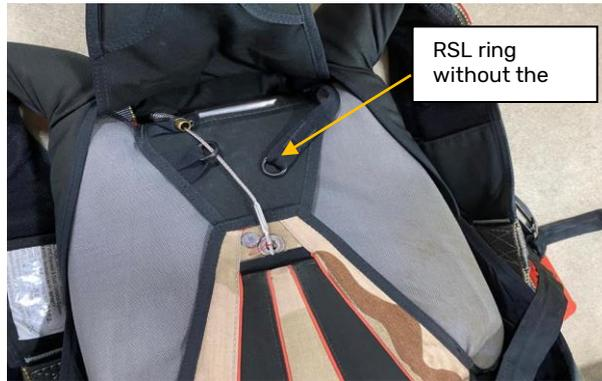
The packer stated that, when packing the reserve, he initially thought the container was not fitted with an RSL, and this was confirmed by marking the Record of Inspection form (ROI) as Non-applicable (N/A). He explained on the report, that he could only think that the RSL ring may have got tucked inside the yoke during the repack, leaving it out of site.
