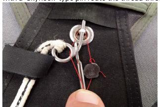
Ensure that the seal cannot fall into the grommet.
