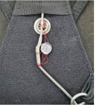
With a 'Skyhook' type pin route the thread through the eye of the pin.
