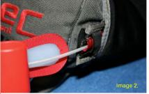
Representation of the plastic tuck-tab handle in a serviceable condition.
