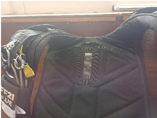
2018 design – Triangle stitching and only about 3/8 inch of material above the back pad binding tape
