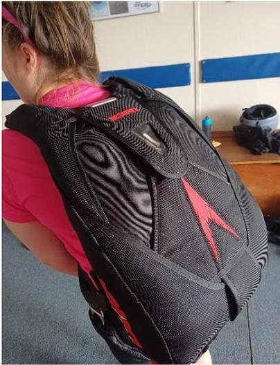
With the 2022 batch we have had a regular issue with the reserve cover flap popping out of the tucked area and then opening in freefall. This can be simulated on the ground by getting the user to roll their shoulder forward. The reserve cover then pops open. This is only evident on the 6 grounded sets of icons.
