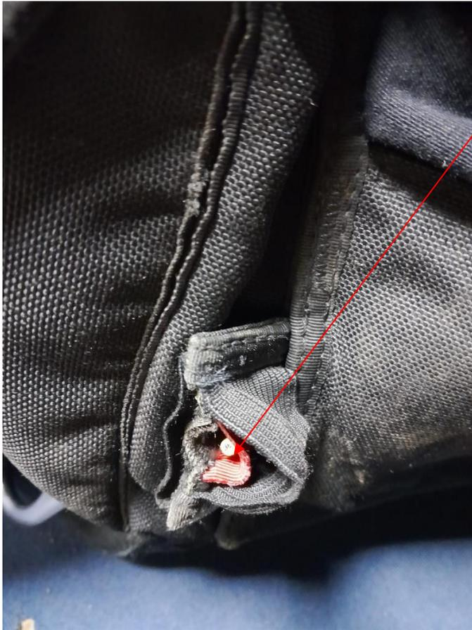
Remaining drogue release cable exposed after handle has sheared off.
