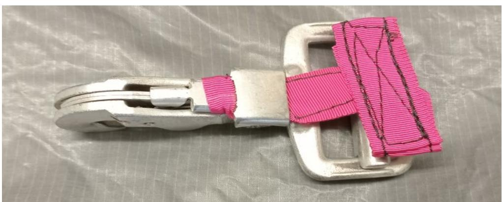
**#2** 15" of type 2a or gutted 550lb line, fingertrapped and knotted, end hot knifed. Open loop to get over the wide part of the lift tab on the buckle, then close tight.
