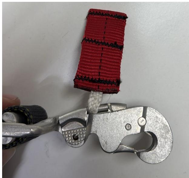
**#5** 6" Spectra finger trapped at  $3\frac{1}{2}$ " and bartacked / zigzagged to  $3\frac{1}{2}$ " type 12 folded in the centre.
